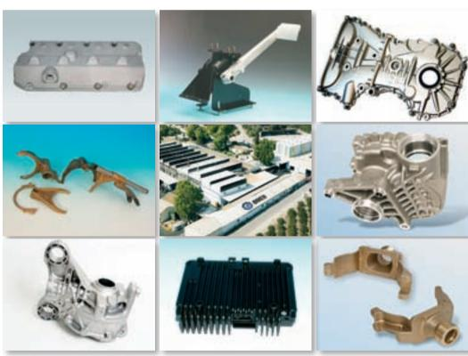
• Fire protection: Automatic brass sprinkler frames. OMEN'S machine park consists of SC Buhler real-time controlled horizontal cold chamber machines with a closing force range of 530–1400 metric tons and sophisticated online process control systems. These enable OMEN the manufacturing of parts ranging from 0.1 Kg and up to 12 Kg.
